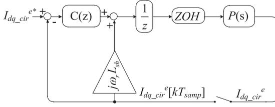
Fig. 8. Complex vector block diagram of the proposed synchronous current controller.
