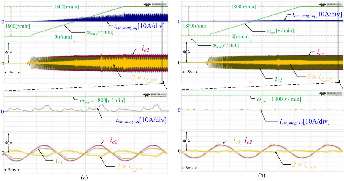
Fig. 13. Experimental results: Acceleration mode under no load condition. (a) Without circulating current suppression control. (b) With circulating current suppression control.
