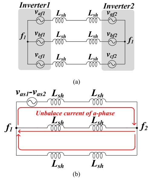
Fig. 2. Circulating current when isolated inverters operating in parallel. (a) Parallel path of 2 parallel operation of non-isolation type. (b) Unbalance current of a-phase.
