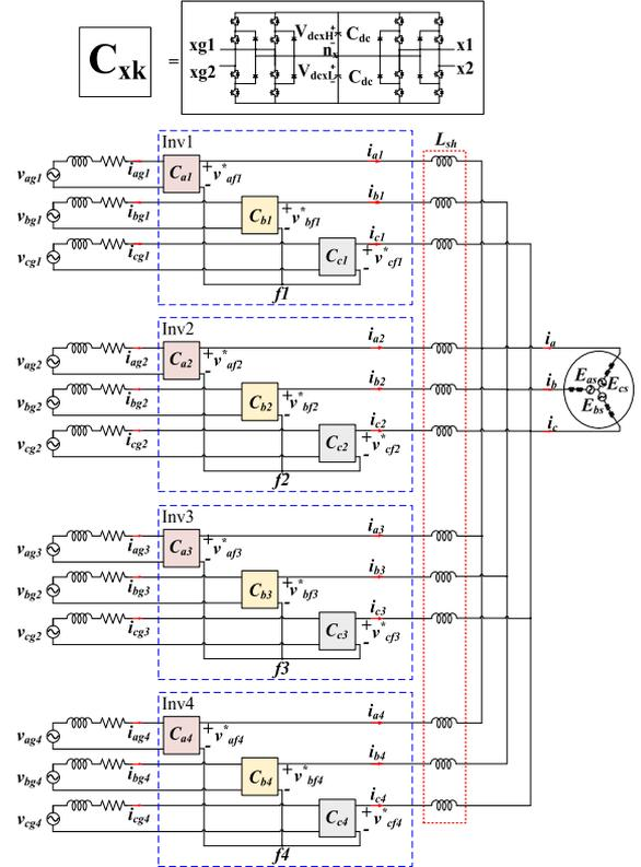
Fig. 10. Simulation model: Four parallel AFE 5L-CHB.
