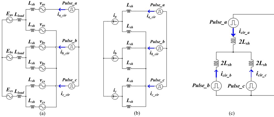
Fig. 4. Equivalent circuit of circulating current. (a) Equivalent circuit including the pulse voltage. (b) Simplified equivalent circuit. (c) Circulating current and pulse voltage model.
