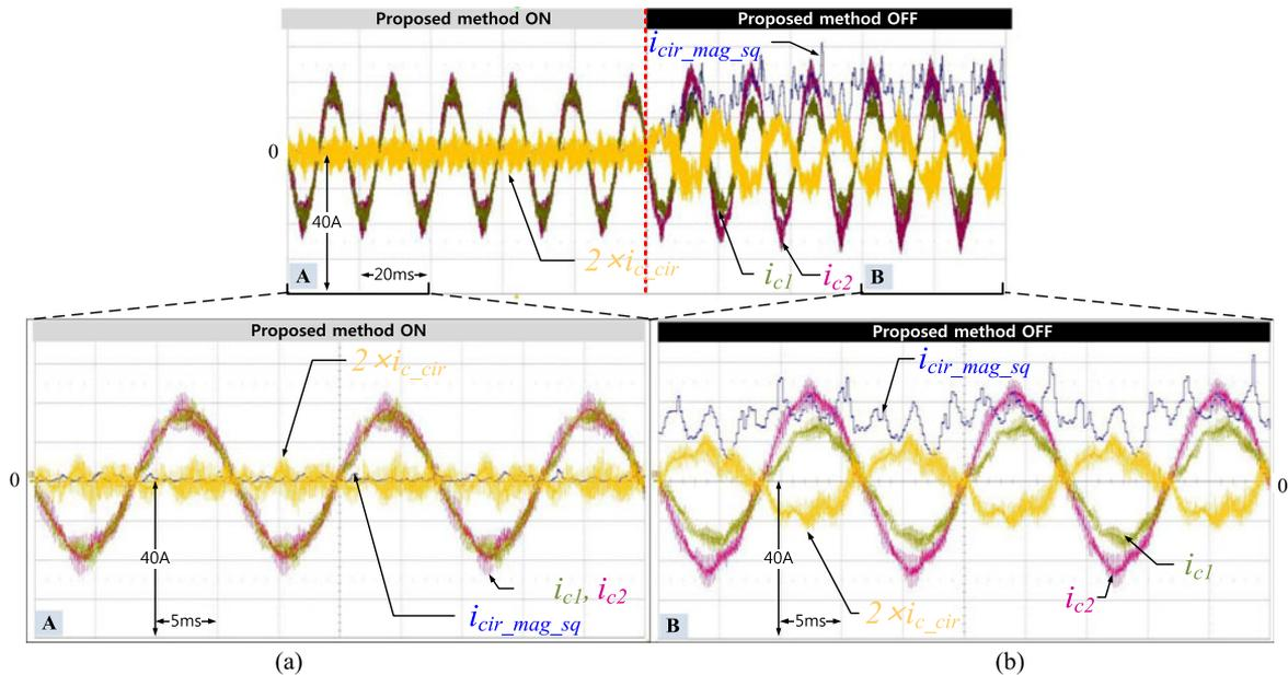
Fig. 14. Experimental results 2: steady state under 75% load condition at rated speed. (a) Expanded waveform with proposed method. (b) Expanded waveform without proposed method.
