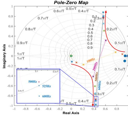
Fig. 9. Complex vector root locus of closed loop with the proposed controller according to its control bandwidth in the  $z$ -domain.
