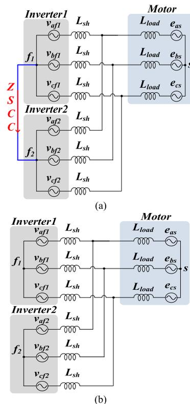
Fig. 1. Type of parallel operation. (a) Non-isolation type. (b) Isolation type.
