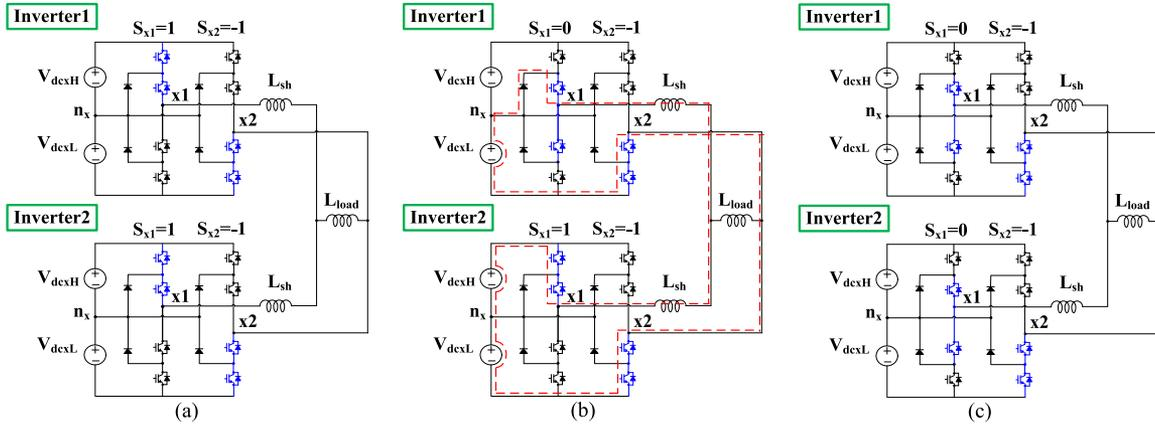
Fig. 3. Example of circulating current provoked by changing switching state asynchronously. (a) Synchronous switching state (start state). (b) Asynchronous switching state. (c) Synchronous switching state (final state).
