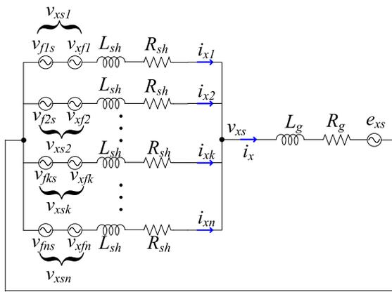
Fig. 5.  $x$ -phase model in  $n$ -paralleled inverters.
