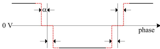
Fig. 13. A-phase pole voltage under OVM3.
