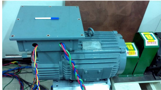
Fig. 11. Experimental setup. (a) Experimental setup. (b) Rotor-side inverter. (c) Test motor; wound-rotor induction motor.
