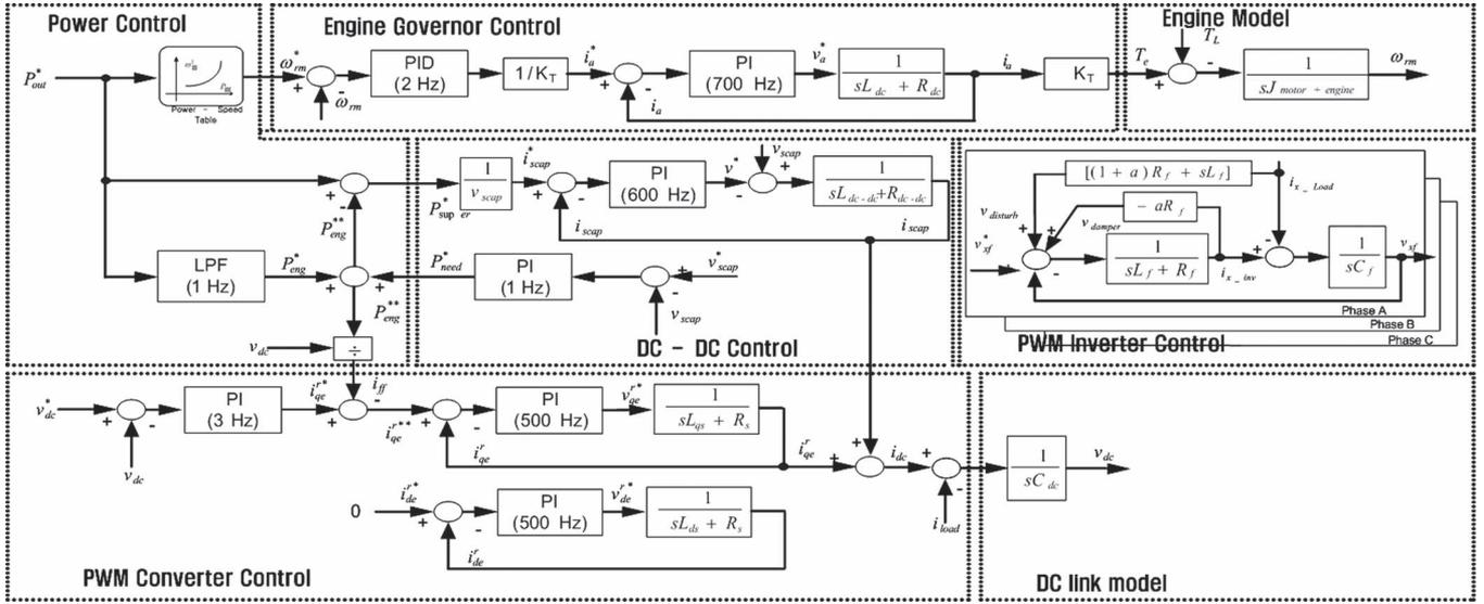
Fig. 3. Block diagram of the overall control system.
