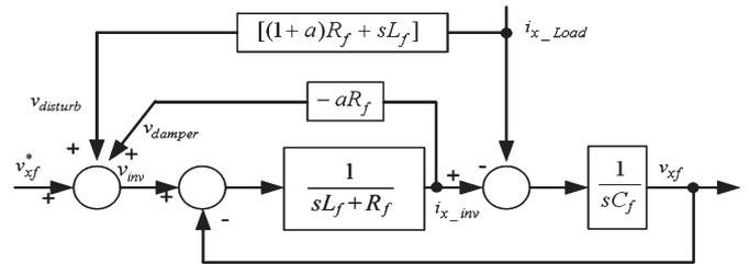
Fig. 5. Control of load disturbance.
