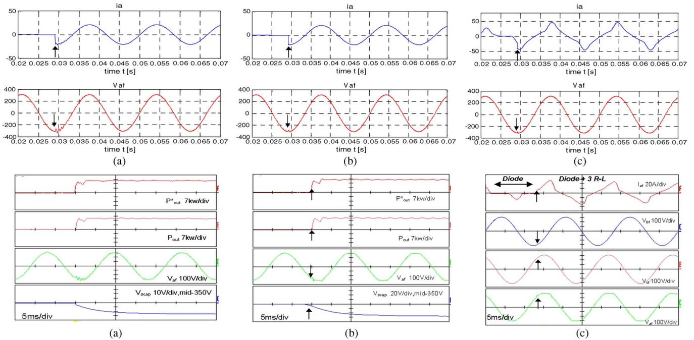
Fig. 7. (Upper) Simulation and (lower) experimental results. (a) *RL* balanced load (20 kW) without a controller. (b) *RL* balanced load (20 kW) with a controller. (c) *RL* balanced load (9 kW) and nonlinear load (2.5 kW) with a controller under mixed load.
