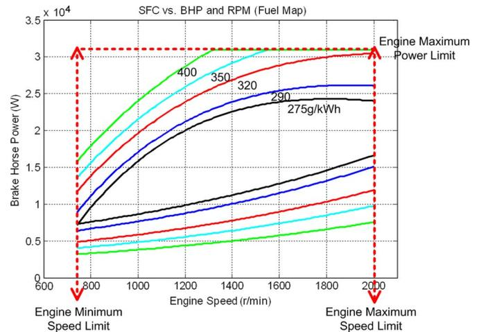
Fig. 1. Experimental results. SFC according to power and speed.
