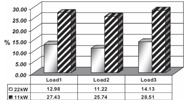
Fig. 10. Saving ratio of fuel consumption.
