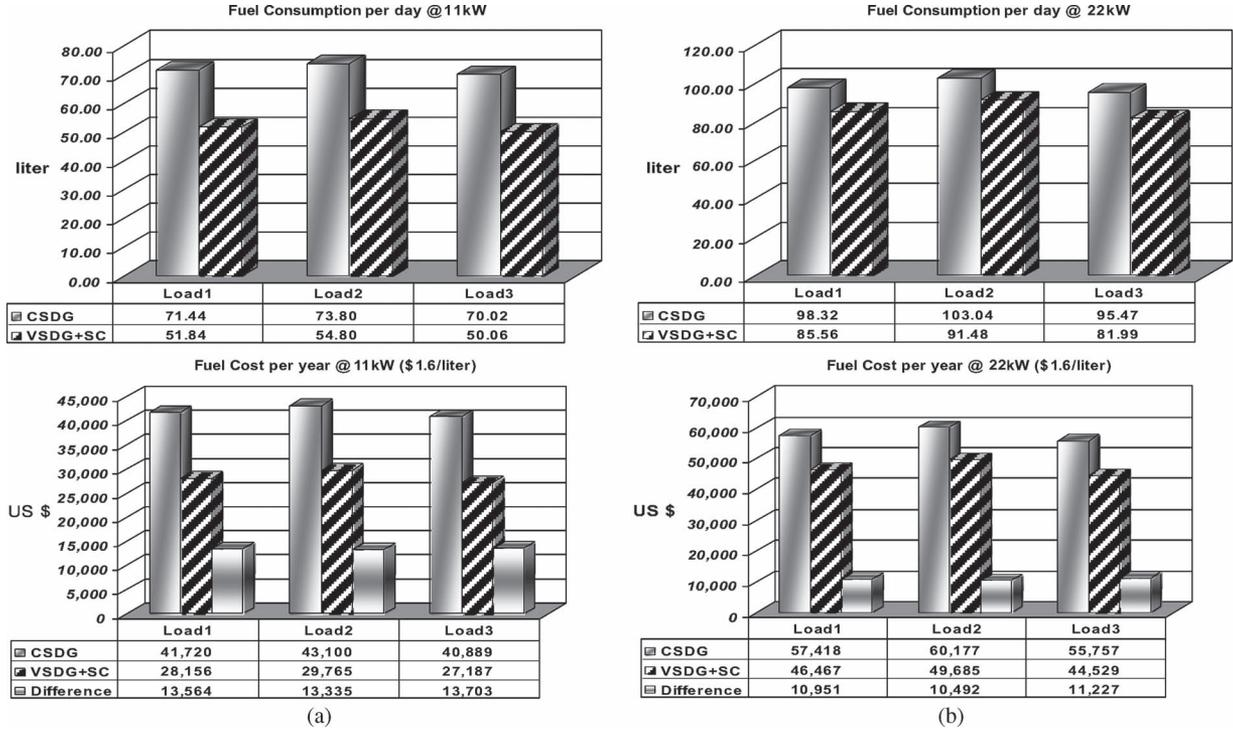
Fig. 9. Comparison of fuel consumption between CSDG and VSDG with an SC. (a) 11 kW. (b) 22 kW.
