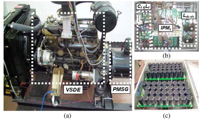
Fig. 6. Hardware structure of the system. (a) VSDE and PMSG. (b) Power stack. (c) SC bank.
