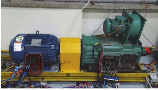
Fig. 15. Motor(left)-Generator(right) set for load test
