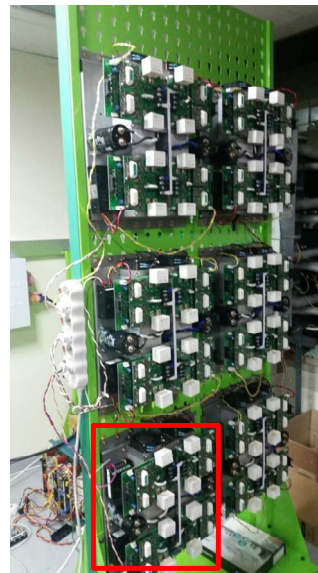
Fig. 14. Single phase back-to-back converter for induction machine drive
