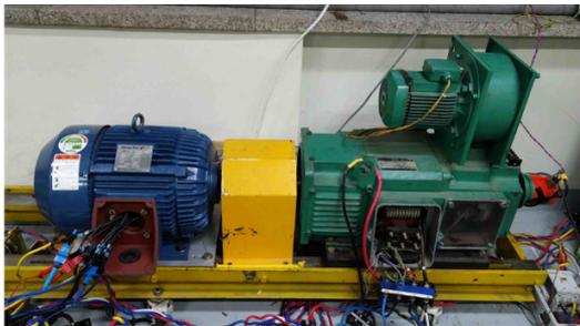
Figure 13. Test set-up for 11 kW DDSW-based induction machine.
