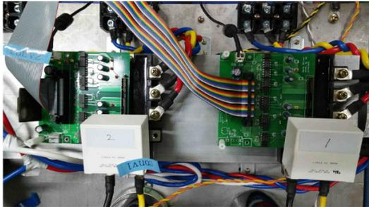
Figure 11. Two-level converters for DDSW.
