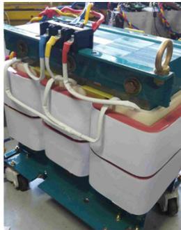
Figure 12. 6 kVA DDSW-based transformer.
