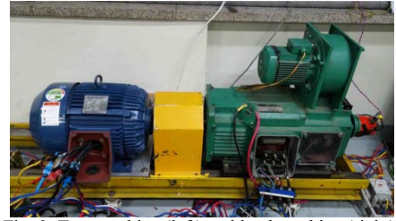
Fig. 9. Test machine (left) and load machine (right).
