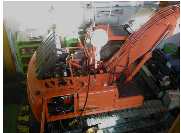
Fig. 10. The compound type hybrid excavator.
