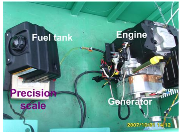
Figure 3. Experimental setup for yielding the SFC map
