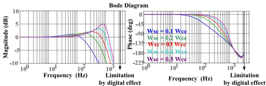
Figure 5 : Bode plot of speed control.
