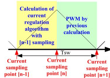
(b) Current sampling at peak and valley of carrier and delay.
