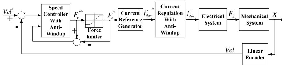
(a) Speed control block diagram of LSM.
