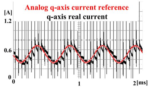
(a) 2[kHz] sinusoidal input.
