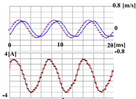
Figure 8 : Speed control performance of the proposed method (300[Hz] input).
