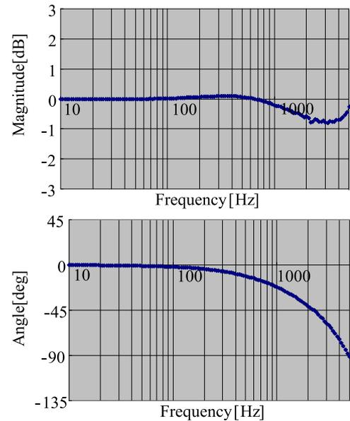
Figure 7 : Bode plot of the proposed current regulator (30[%] offset and 10[%] magnitude of rated current).
