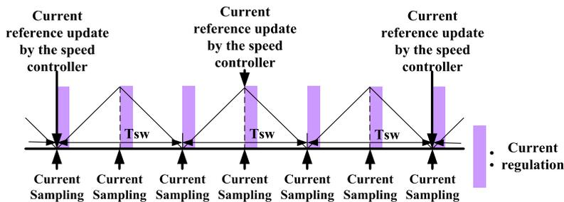
(b) Speed control timing diagram of LSM.
