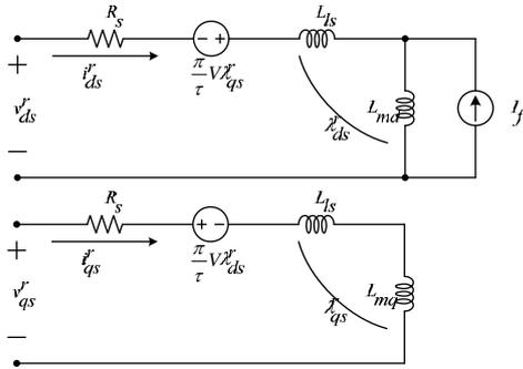
Figure 2 : Equivalent circuit of LSM.
