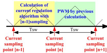
(a) Current sampling at peak or valley of carrier and delay.
