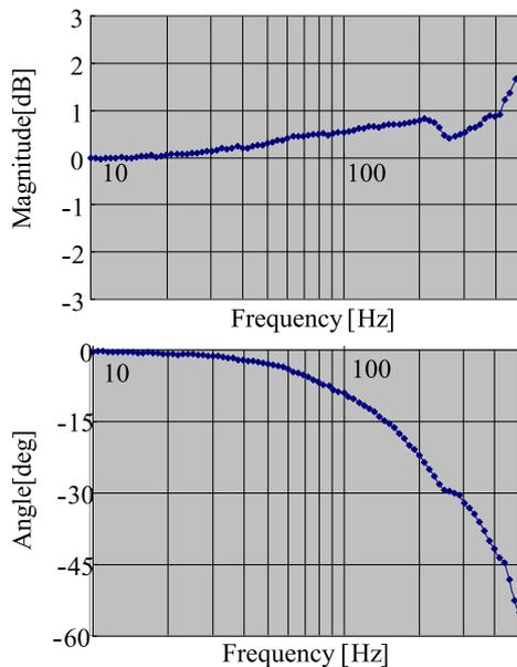
Figure 9 : Bode plot of the speed control with proposed current regulator.
