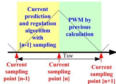
(c) Current sampling at peak and valley of carrier, current prediction and delay.
