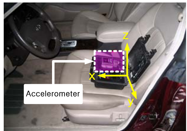
Fig. 15. Position of accelerometer
